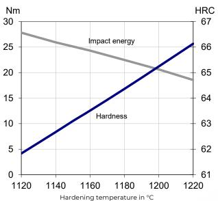
Tempering 3 x 1 hour at 560° C Unnotched test piece 7 x 10 x 55 mm
